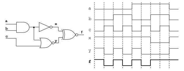
b) Complete the timing diagram of the logic circuit whose VHDL description is shown below:
