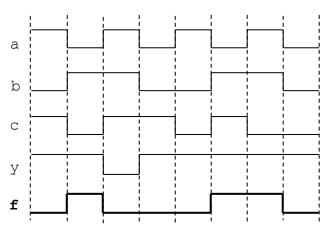
c) The following is the timing diagram of a logic circuit with 3 inputs. Sketch the logic circuit that generates this waveform. Then, complete the VHDL code.
