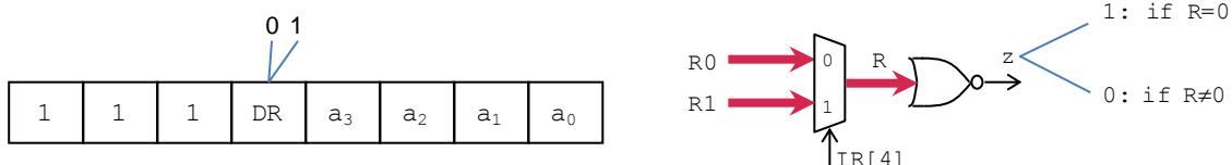
JNZ R0, ADDRESS: 1110a<sub>3</sub>a<sub>2</sub>a<sub>1</sub>a<sub>0</sub>  $\Rightarrow$  M6  $\leftarrow$  0 if z = 1, M6  $\leftarrow$  1 if z = 0
